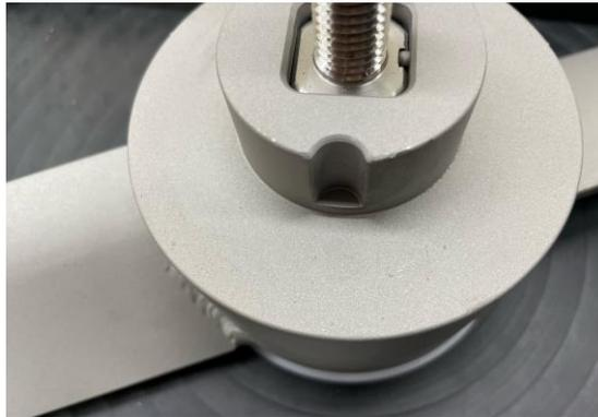
Next position the top paddle over the drive paddle shaft ensuring the paddle pin engages with paddle slot on the bottom paddle. (See image)
