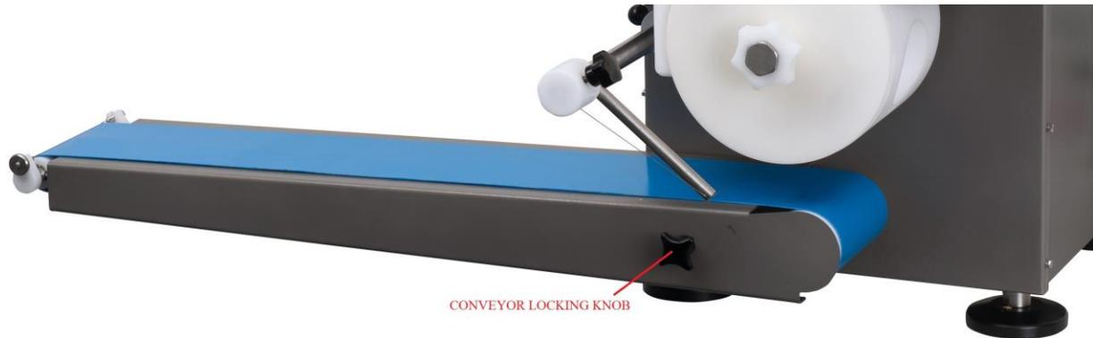
**Wash the belt and platform with hot soapy water, rinse with clean water and allow to dry. Do not use strong alkaline/acid based cleaners.**
