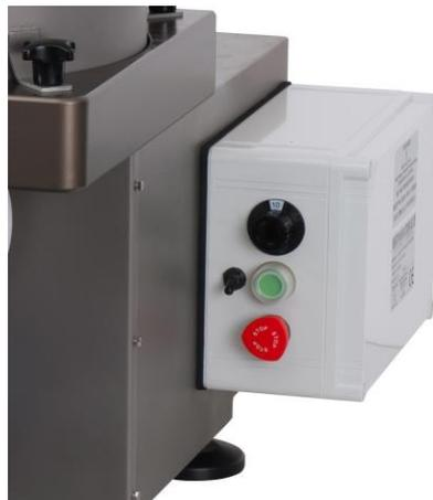
**ALWAYS TRY TO KEEP WATER AWAY FROM THE CONTROL BOX INTERFACE SCREEN AND MOTORS. DO NOT PRESSURE WASH.**
