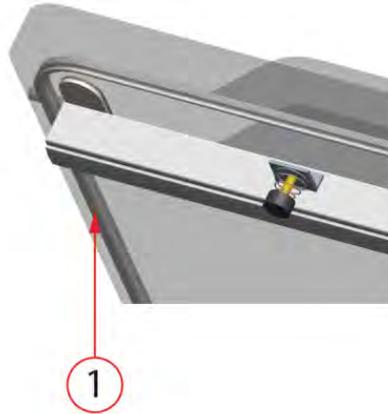
Figure 9: Replacing the Lid Gasket
