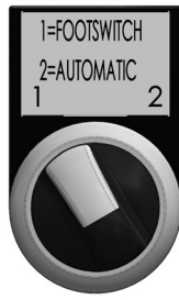
Figure 24: Automatic lid switch
