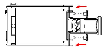
❖Tighten the two clamp handles setting the body on the machine.
