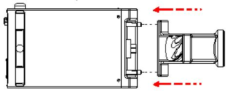
❖ Fit the body in its seat (two bolts through).
